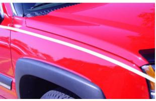
4. If necessary, lift the masking tape and reposition as needed if you don't lay it into a satisfactory position on the first attempt. Step back to view the overall placement of the tape. Adjust as needed.
