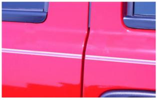
6. Trim stripe about 1/8" from all door edges, using light knife pressure when cutting. Trim ends of the stripe as desired. Remove masking tape, and repeat on the other side.
