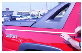
1. Determine placement of the pinstripe by using a line of masking tape as a guide. Start from the rear quarter panel and tack one end of the masking tape to the vehicle.
