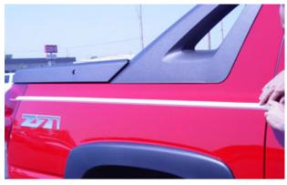
5. Lay the stripe along the bottom edge of the masking tape. Once in position, press firmly with your thumb or a squeegee along the entire stripe. Now peel back the clear premask at a 180 angle from the application surface.
