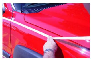
3. On the front fender, the stripe application may need to flow down at an angle toward the headlight. Align your masking tape with the top edge of the front fender, and lightly tack the masking tape into position.
